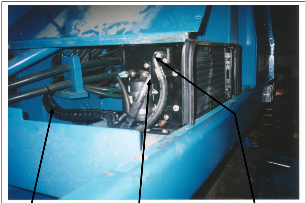
Hoses and wiring continuing towards the electric condenser.
